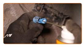
19 Attach the ABS sensor connector.
