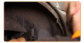
Install and tighten the wheel arch cover fasteners. Use a drive socket #10. Use a ratchet wrench.
