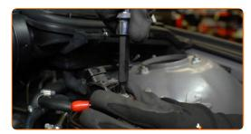
Attach the tubes to the fuel filter.
