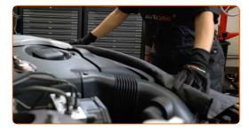
Detach the fuel pressure sensor connector.
