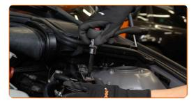
Remove the fuel pressure sensor.
