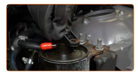
Screw the fastener of the fuel pressure sensor. Use Torx T50. Use a ratchet wrench.
