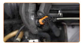
Attach the fuel pressure sensor connector.
