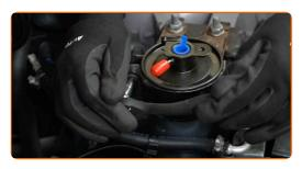
12 Install the fuel pressure sensor.
