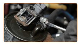
Treat the fuel pressure sensor connector. Use dielectric grease.
