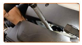
27 Install the fan shroud clips.
