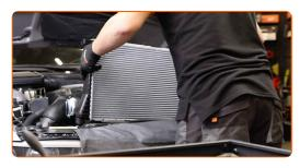
Screw in the radiator fasteners. Use a drive socket #8. Use a ratchet wrench.
