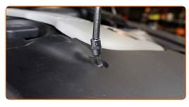
Remove the fender protection cover.
