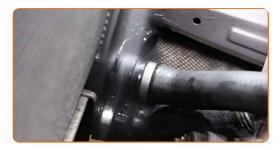
Attach the lower coolant pipe.
