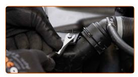
Unscrew the cooling fan fastener. Use a combination spanner #32 (2 pieces).
