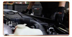
Unscrew the coolant reservoir cap.
