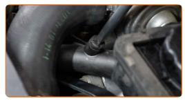
Remove the coolant reservoir cap.
