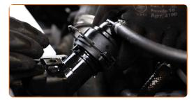
Attach the clamp of the upper coolant hose.
