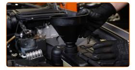
Pour coolant in the coolant reservoir.
