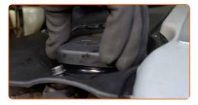
Screw in the engine cover fasteners. Use HEX No.H5. Use a ratchet wrench.
