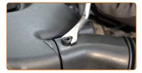
Detach the air duct housing from the air filter housing. Use a clip removal tool.
