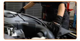
Unscrew the engine cover fastener. Use HEX No.H5. Use a ratchet wrench.
