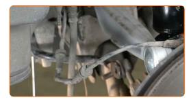
Remove the support from under the arm.
