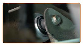
Screw in the fastener that connects the control arm to the rear knuckle. Use a combination spanner #22. Use a drive socket #10. Use a ratchet wrench.
