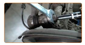
Unscrew the arm fastening to the beam. Use a combination spanner #16.
