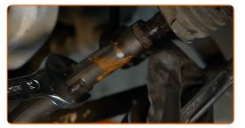
17 When deinstalling, mark or measure the precise position of the ball joint on the track rod, or count the number of turns in order to prevent misalignment afterward. Use a vernier caliper.
