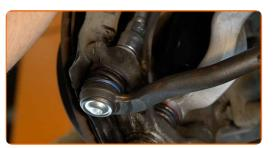
20 Tighten the tie rod end locknut. Use a combination spanner #24 (2 pieces). Use a torque wrench. Tighten it to 51 nm torque.
