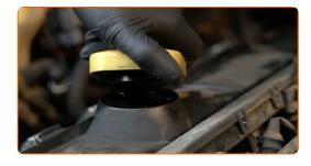
25 Install the engine cover and secure it.
