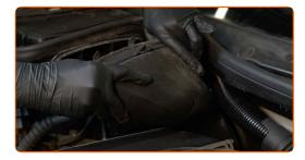
Unscrew the engine cover fastener. Use a drive socket #10. Use a ratchet wrench.
