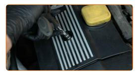
29 Install the air duct housing.
