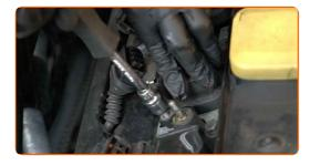
Tighten the ignition coil fasteners. Use a drive socket #10. Use a torque wrench. Tighten it to 11 nm torque.
