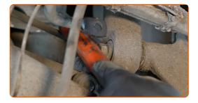
Unscrew the lower fastener of the shock absorber strut. Use a drive socket #21. Use a tap wrench.
