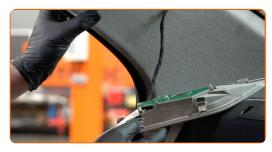
6 Unscrew the rear seat headrest bracket. Use a Phillips screwdriver.
