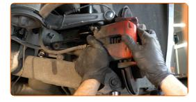
72 Tighten the brake caliper bracket. Use a drive socket #16. Use a torque wrench. Tighten it to 65 Nm torque.
