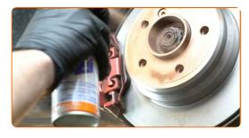
79 Clean the brake disk surface. Use a brake cleaner.
