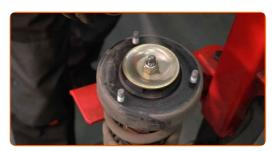
Remove the strut piston rod nut. Use a shock absorber socket DDNº6. Use a drive socket #16. Use a ratchet wrench.
