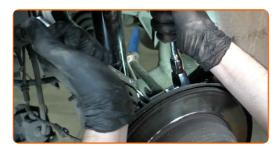
Tighten the fastener connecting the suspension arm to the rear knuckle. Use a drive socket #22. Use a torque wrench. Tighten it to 142 Nm torque.
