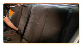
Screw in the fasteners of the rear seat backrest. Use a drive socket #10. Use a ratchet wrench.
