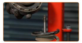
Release the coil spring.
