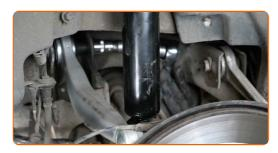
Connect the ABS sensor wiring.
