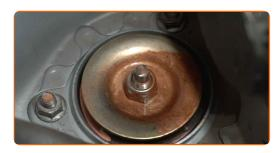
86 Install the shock strut mount cap.
