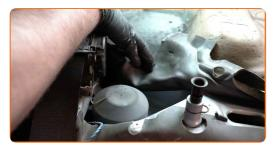
Remove the shock strut mount cap.
