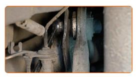
Detach the bottom part of the shock strut. Use a crowbar.
