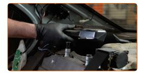
Bend the interior sound insulation upwards.
