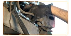
73 Connect the brake pads wear sensor.
