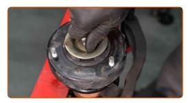
Tighten the shock strut piston rod nut. Use a shock absorber socket DDNº6. Use a drive socket #16. Use a torque wrench. Tighten it to 27 Nm torque.
