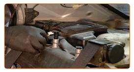
Screw in the fasteners of the speakers. Use a Phillips screwdriver.
