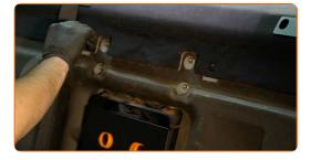
Screw in the rear seat headrest bracket. Use a Phillips screwdriver.
