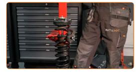
Remove the assembled shock strut.
