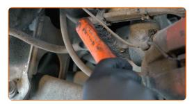
Unscrew the fastener connecting the stabilizer link to the stabilizer bar. Use a combination spanner #16. Use a drive socket #16. Use a ratchet wrench.
