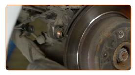
Remove the fastening bolt.
