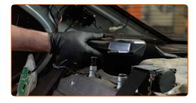
Bend the interior sound insulation upwards.
