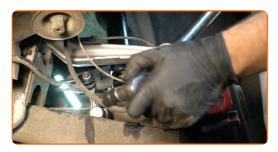
Treat all joints of the arm. Treat the shock strut fasteners. Use copper grease. 79
