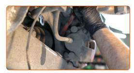
Unscrew the caliper bracket fastening. Use a drive socket #16. Use a tap wrench.
