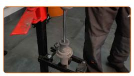
Remove the old shock absorber from the hydraulic coil spring compressor.
