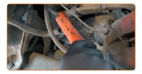
Unscrew the fastener connecting the stabilizer link to the stabilizer bar. Use a combination spanner #16. Use a drive socket #16. Use a ratchet wrench.
