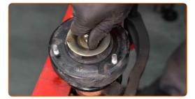
Tighten the shock strut piston rod nut. Use a shock absorber socket DDNº6. Use a drive socket #16. Use a torque wrench. Tighten it to 27 Nm torque.
