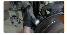
Screw in the fastener that connects the control arm to the rear knuckle. Use a combination spanner #22. Use a drive socket #10. Use a ratchet wrench.
