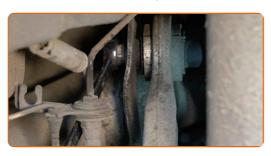
Detach the bottom part of the shock strut. Use a crowbar.
