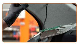
6 Unscrew the rear seat headrest bracket. Use a Phillips screwdriver.
