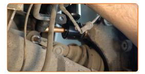
Tighten the lower fastening of the shock absorber. Use a drive socket #21. Use a torque wrench. Tighten it to 127 Nm torque.
