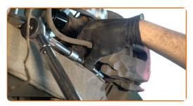
Connect the brake pads wear sensor.
