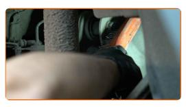
Disconnect the ABS sensor wiring.
