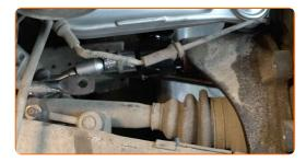
Tighten the arm fastening to the beam. Use a drive socket #16. Use a torque wrench. Tighten it to 110 nm torque.
