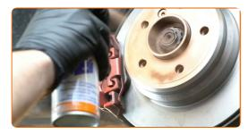
Clean the brake disk surface. Use a brake cleaner. 81
