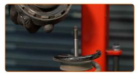
Release the coil spring.
