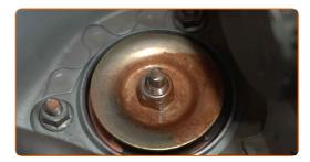
Install the shock strut mount cap.
