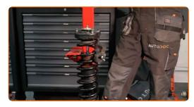
Remove the assembled shock strut.
