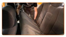
Unscrew the fasteners of the rear seat backrest. Use a drive socket #10. Use a ratchet wrench.
