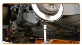
Screw in the fastener connecting the control arm to the subframe. Use a combination spanner #16.
