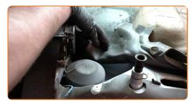
Remove the shock strut mount cap.
