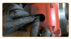
Install the brake caliper retaining spring.
