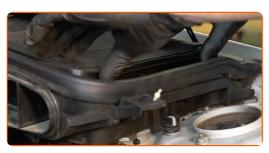
Install the air duct housing.
