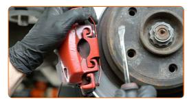
19 Remove the brake caliper.
