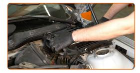
Reinstall the cabin filter housing seal.
