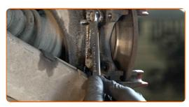
Remove the caliper bracket.
