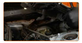
8 Unscrew the brake fluid reservoir cap.
