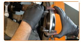
Tighten the brake caliper bracket. Use a drive socket #16. Use a torque wrench. Tighten it to 65 Nm torque.
