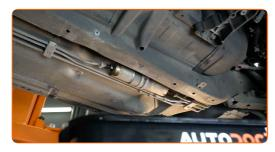
Unscrew the fastener attaching the fuel supply line to the fuel filter housing. Use a drive socket #5.5. Use a ratchet wrench.
