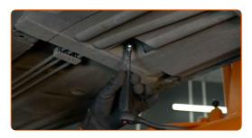
Remove the clips of the underbody cover panel. Use a clip removal tool.
