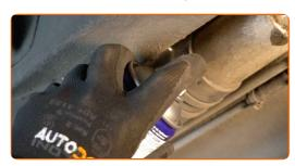
Loosen the fuel filter mounting. Use HEX No.H5. Use a ratchet wrench.
