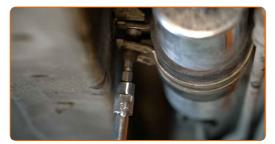
Screw the fastener attaching the fuel supply line to the fuel filter housing. Use a drive socket #5.5. Use a ratchet wrench.
