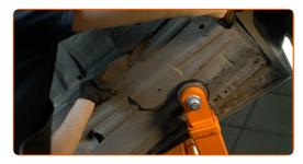
Screw in the fasteners of the underbody cover panel. Use a drive socket #8. Use a drive socket #10. Use a ratchet wrench.
