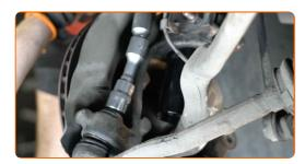
Remove the support from under the arm.
