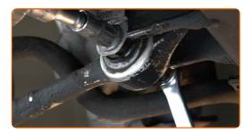
Screw the front arm fastener. Use a combination spanner #18. Use a drive socket #18. Use a ratchet wrench.
