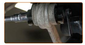
Tighten the front fastener connecting the control arm to the subframe. Use a combination spanner #18. Use a drive socket #18. Use a torque wrench. Tighten it to 110 Nm torque.
