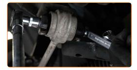
Tighten the rear fastener connecting the arm to the body subframe. Use a combination spanner #16. Use a drive socket #18. Use a torque wrench. Tighten it to 110 nm torque.
