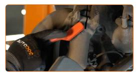
Release the lower fastener connecting the shock strut to the steering knuckle. Use a special drive socket to remove the shock absorber.
