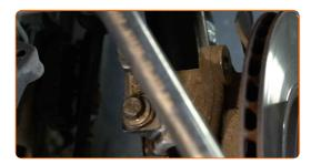
Tighten the fastening nut connecting the tie rod end to the steering knuckle. Use a drive socket #18. Use a torque wrench. Tighten it to 65 nm torque.
