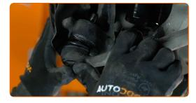
Screw on the fastening nut that connects the tie rod end to the steering knuckle. Use a combination spanner #18.
