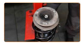
Tighten the shock strut piston rod nut. Use a drive socket #22. Use HEX No.H6. Use a torque wrench. Tighten it to 64 Nm torque.
