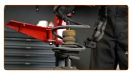
Remove the shock absorber dust cap and the bump stop.
