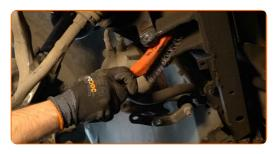
Install the rear fastener of the control arm.
