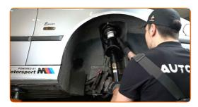
Screw the top fastening of the shock strut mount. Do not tighten it.
