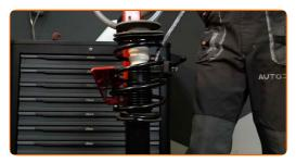
Remove the assembled shock strut.
