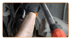
Tighten the fastener connecting the stabilizer link to the stabilizer bar. Use a drive socket #17. Use a torque wrench. Tighten it to 65 Nm torque.
