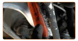
Unscrew the fastener connecting the stabilizer link to the stabilizer bar. Use a drive socket #17. Use a ratchet wrench.
