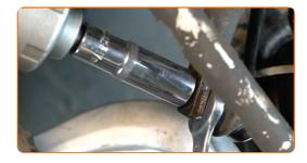
Tighten the fastener connecting the stabilizer link to the shock strut. Use a drive socket #17. Use a torque wrench. Tighten it to 65 Nm torque.
