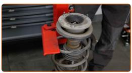
Remove the strut piston rod nut. Use a drive socket #22. Use HEX No.H7. Use a ratchet wrench.
