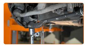
Screw the rear fastener connecting the control arm to the subframe. Use a combination spanner #16. Use a drive socket #18. Use a ratchet wrench.
