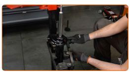
Install the dust sleeve and the bump stop on the new shock absorber.
