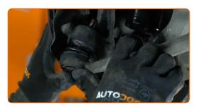
Screw on the fastening nut that connects the tie rod end to the steering knuckle. Use a combination spanner #18.
