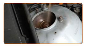
97 Install the shock strut mount cap.
