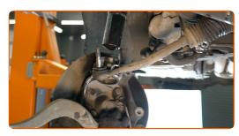
Unscrew the top fastening of the shock strut mount.
