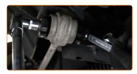
Tighten the rear fastener connecting the arm to the body subframe. Use a combination spanner #16. Use a drive socket #18. Use a torque wrench. Tighten it to 110 nm torque.
