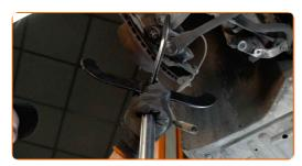
Unscrew the rear fastener connecting the control arm to the subframe. Use a combination spanner #16. Use a drive socket #18. Use a ratchet wrench.
