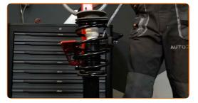
Remove the assembled shock strut.
