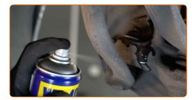
Unscrew the end fastening nut to the steering knuckle. Use a combination spanner #18.
