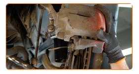
Tighten the brake caliper bracket. Use a drive socket #18. Use a torque wrench. Tighten it to 110 Nm torque.
