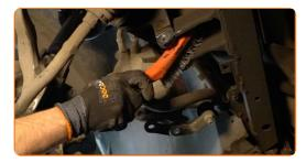
Install the rear fastener of the control arm.
