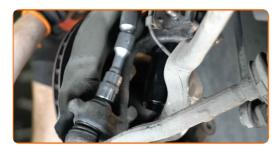
Remove the support from under the arm.
