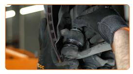
70 Install the shock absorber mount using the center hole as a guide.
