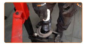
Install the spring on the shock absorber.
