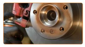
90 Clean the brake disk surface. Use a brake cleaner.
