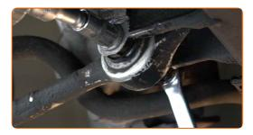
Screw the front arm fastener. Use a combination spanner #18. Use a drive socket #18. Use a ratchet wrench.
