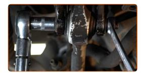
Tighten the lower fasteners connecting the shock strut to the steering knuckle. Use a combination spanner #18. Use a drive socket #16. Use a torque wrench. Tighten it to 81 Nm torque.
