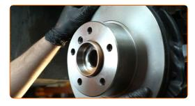
Tighten the brake disc fastening. Use HEX No.H6. Use a torque wrench. Tighten it to 16 Nm torque.
