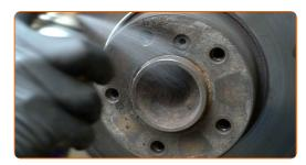
Unscrew the brake disc fastening. Use HEX No.H6. Use an impact screwdriver.
