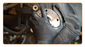
Tighten the hub. Use a drive socket #18. Use a torque wrench. Tighten it to 110 Nm torque.
