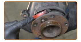
Unscrew the wheel hub axle nut. Use a combination spanner #18.
