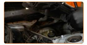
8 Unscrew the brake fluid reservoir cap.
