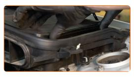
38 Install the air duct housing.
