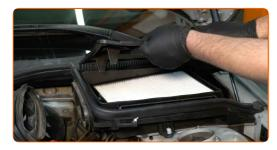
6 Remove the cabin filter housing seal.
