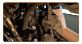
27 Install the brake caliper retaining spring.
