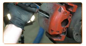
Detach the brake caliper retaining spring. Use a crowbar.
