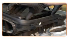
Install the air duct housing.
