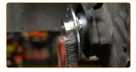
Treat the contacting surface. Use copper grease.
