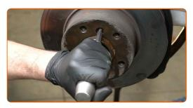
Remove the brake disc.
