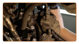
Install the brake caliper retaining spring.
