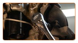
Remove the caliper bracket.
