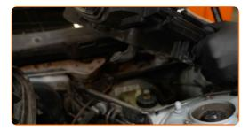
8 Unscrew the brake fluid reservoir cap.
