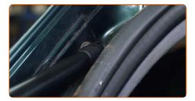
Snap on the circlip connecting the gas strut to the boot lid.
