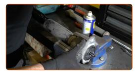
Tighten the shock absorber rod nut. Use a shock absorber socket DD№6. Use a combination spanner #17. Use a torque wrench. Tighten it to 25 nm torque.
