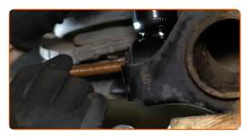
Tighten the lower fastener of the shock absorber. Use a combination spanner #16. Use a drive socket #16. Use a torque wrench. Tighten it to 50 Nm torque.+90°
