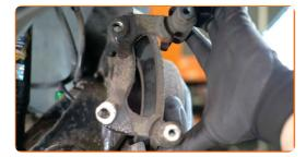
14 Remove the brake disc.
