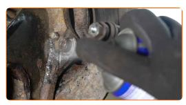
Unscrew the caliper bracket fastening. Use HEX No.H8. Use a tap wrench. Use a ratchet wrench.
