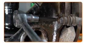
13 Remove the caliper bracket.
