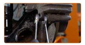
Remove the brake caliper. Use a crowbar.
