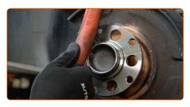
16 Install the brake disc.
