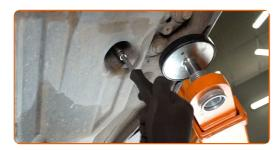
6 Remove the plastic car body protective cover.
