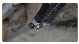
18 Attach the tubes to the fuel filter.
