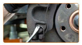
Remove the brake caliper.
