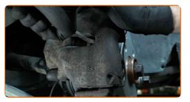
Clean the area where the brake hose is connected to the caliper, and the guide pins area. Use a wire brush. Use a brake cleaner.
