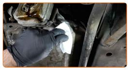
Screw in the new oil drain plug.
