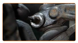
Loosen the tie rod end fastening bolt. Use a drive socket #13. Use a ratchet wrench.
