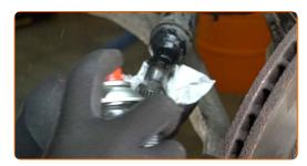
Remove the CV joint circlip. Use a flat screwdriver.
