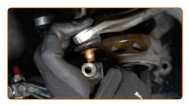
Install the fastening bolt. Use a crowbar.
