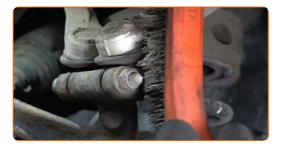
Unscrew the upper arm fastenings. Use a drive socket #16. Use HEX No.H8. Use a ratchet wrench.
