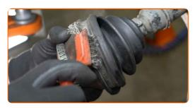
Detach the clamps of the CV joint boot. Use a flat screwdriver.
