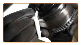
Install the boot on the CV joint.
