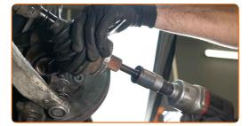
Remove the fastening bolt.
