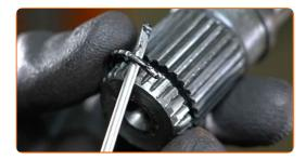
Install the CV joint boot on the CV axle. Use a flat screwdriver.
