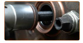
Detach the driveshaft from the steering knuckle.
