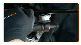
Screw in the fasteners of the upper control arms. Use a drive socket #16. Use HEX No.H8. Use a ratchet wrench.
