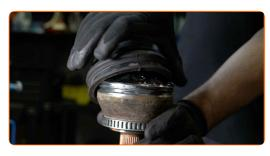
Clean the CV joint mounting seat. Use all-purpose cleaning spray.
