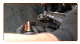
Remove the fastening bolt. Use a drive socket #27.
