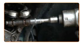
Tighten the upper arm fastenings. Use a drive socket #16. Use HEX No.H8. Use a torque wrench. Tighten it to 40 Nm torque.
