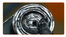
Install the new CV joint. Use a bush and bearing driver set. Use a hammer.
