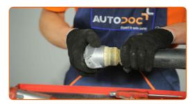
Screw the shock strut piston rod upper fastening. Use a drive socket #16. Use a torque wrench. Tighten it to 25 nm torque.
