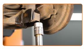
9 Remove the fastening bolt.
