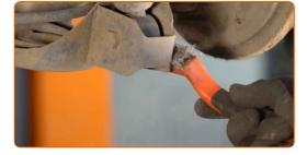
Unscrew the lower fastener of the shock absorber. Use a combination spanner #16. Use a drive socket #16. Use a ratchet wrench.
