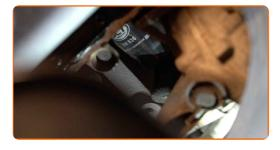
9 Unscrew the oil filter. Use a drive socket #30. Use a ratchet wrench.
