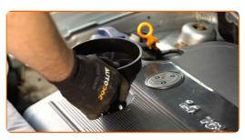
Pour oil into the engine through the filler. Required amount of oil: 3.2 l.
