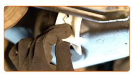
Screw in the new drainage plug and tighten it. Use a drive socket #19. Use a torque wrench. Tighten it to 30 Nm torque.
