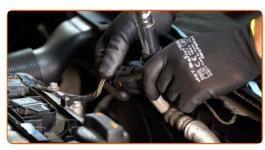
Install the new ignition coil to the spark plug well. Make sure you hear a click indicating that it is locked in place.
