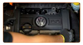
Undo the plastic locking tabs of the ignition coil connector.
