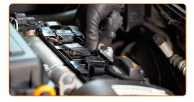
Install the engine cover and secure it. Use Torx T30. Use a torque wrench. Tighten it to 10 Nm torque.
