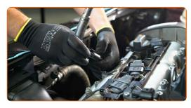
Treat the ignition coil tip. Use high-temperature grease.
