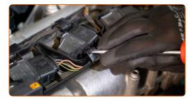
Pry up the ignition coil. Use a flat screwdriver.
