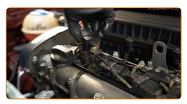
9 Detach the connector from the ignition coil.
