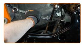
Tighten the fastening nut connecting the tie rod end to the steering knuckle. Use a drive socket #19. Use a torque wrench. Tighten it to 48 nm torque.
