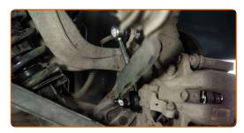
Tighten the fastener connecting the stabilizer bar with the control arm. Use a combination spanner #16. Use Torx T30. Use a torque wrench. Tighten it to 40 Nm torque.
