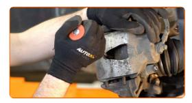
Remove the brake caliper.
