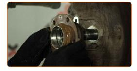
Install the new wheel hub with a bearing. Use a rubber mallet.
