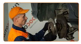
Remove the hub bearing protection cap. Use a crowbar. Use a hammer.
