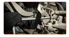
Remove the caliper bracket.
