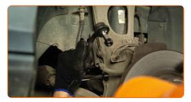
Tighten the fastener connecting the stabilizer link to the stabilizer bar. Use a combination spanner #18. Use HEX No.H6. Use a torque wrench. Tighten it to 85 Nm torque.
