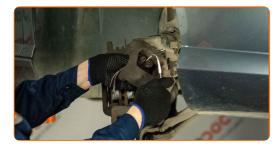
Connect the brake pad wear sensor cable.
