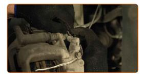
Connect the brake pad wear sensor plug.
