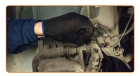
Disconnect the brake pad wear sensor cable. Use a flat screwdriver.
