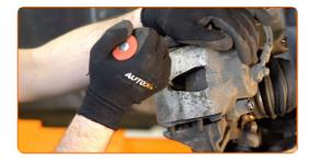
Remove the brake caliper.
