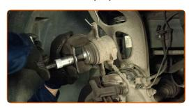
Install the brake caliper and fix it. Use a combination spanner #15. Use a drive socket #13. Use a torque wrench. Tighten it to 30 Nm torque.
