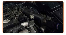
Cover the turbocharger impeller with a microfibre cloth, to prevent the ingress of dirt and foreign objects into the system.
