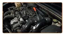
Remove the air distribution housing assembly. Use a flat screwdriver.
