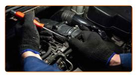
9 Undo the fastening screws of the air filter cover. Use a Phillips screwdriver.
