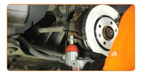
Tighten the tie rod end locknut. Use a combination spanner #24. Use a torque wrench. Tighten it to 60 nm torque.
