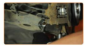
Remove the fastening bolt.
