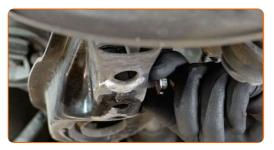
Remove the support from under the rear control arm.
