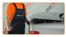
Remove the clips of the boot side lining. Use a clip removal tool.
