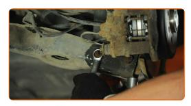
9 Remove the fastening bolt.
