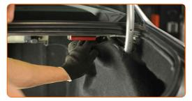
Install the clips of the boot side lining.
