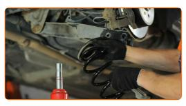
Install the coil spring together with the rubber mounts into the mounting seats.
