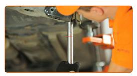
Tighten the fastener connecting the control arm to the rear knuckle. Use a combination spanner #21. Use a drive socket #21. Use a torque wrench. Tighten it to 95 Nm torque.
