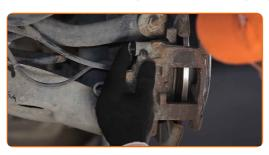
Install the brake pads. Use a crowbar.
