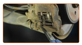
Remove the brake pads retaining clips. Use a pin punch. Use a hammer.
