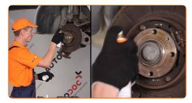
19 Install the brake disc.
