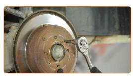
17 Remove the brake disc.
