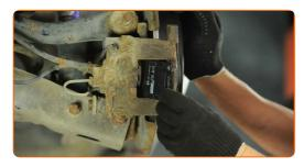
Install the brake pads retaining clips. Use a crowbar. Use a hammer.
