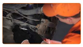
14 Remove the brake caliper.
