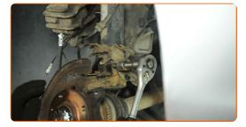
66 Connect the ABS sensor wiring.
