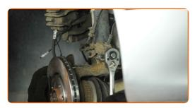
Remove the bracket from the suspension strut.
