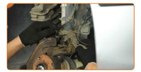
Tighten the ABS sensor wiring bracket. Use a drive socket #10. Use a torque wrench. Tighten it to 10 Nm torque.
