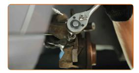
Remove the ABS sensor from the steering knuckle.
