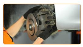
73 Treat the brake caliper bracket fasteners. Use a sealant.
