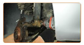
Treat the splines of the driveshaft CV joint. Use a wire brush. Use WD-40 spray.
