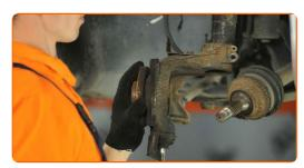
Unscrew the fastener connecting the ABS sensor to the steering knuckle. Use a drive socket #10. Use a ratchet wrench.
