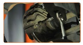
Connect the brake pad wear sensor plug.
