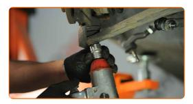
Disconnect the lower control arm from the steering knuckle. Use a ball joint puller. Use a crowbar.
