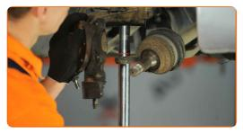
Fix the shock absorber strut on the steering knuckle. Use a hammer.
