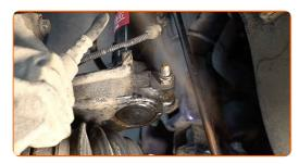
78 Treat the surface where the brake disc contacts the wheel rim. Use high-temperature ceramic grease.
