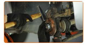
Install the ABS sensor on the steering knuckle and secure it. Use a drive socket #10. Use a ratchet wrench.
