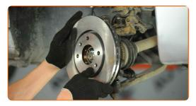
Tighten the brake disc fasteners. Use a Phillips screwdriver. Use a torque wrench. Tighten it to 10 Nm torque.
