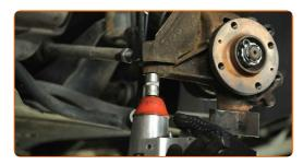
Install the bracket on the suspension strut.
