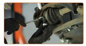
Remove the cotter pin securing the hub nut. Use round-nose pliers. Use a flat screwdriver.
