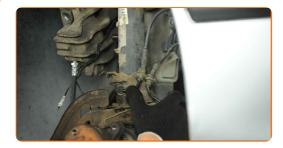
Attach the brake hose retainer clip.
