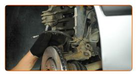
Disconnect the ABS sensor wiring. Use a crowbar.
