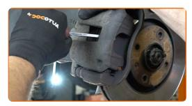
Remove the brake caliper. Use a crowbar.
