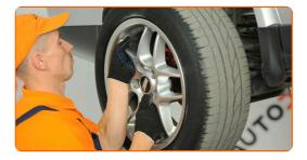
Disconnect the parking brake cable from the caliper. Use a flat screwdriver.
