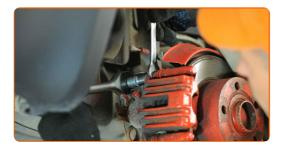
Remove the brake caliper. Use a flat screwdriver.
