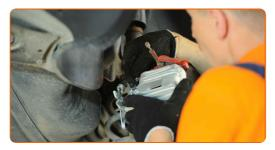
Secure the parking brake cable with the retaining clip. Use a flat screwdriver.
