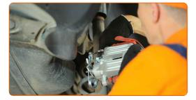
Undo the brake bleeder screw. Use a flare nut spanner #10.
