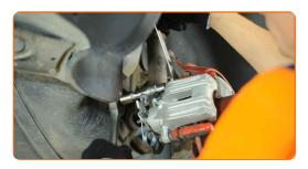
Install the parking brake cable into the brake caliper bracket. Use a flat screwdriver.
