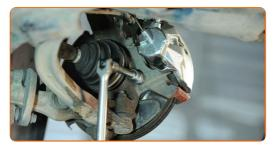
Disconnect the ABS sensor electric socket. Use a flat screwdriver.
