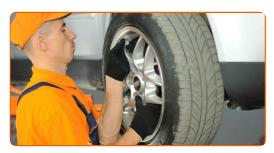
Unscrew the wheel hub axle nut. Use a drive socket #27.
