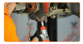
Tighten the ball joint fastener. Use a drive socket #18. Use a torque wrench. Tighten it to 100 Nm torque.
