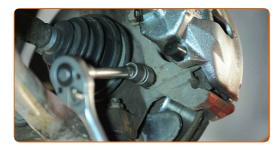
50 Connect the ABS sensor cable fastener.
