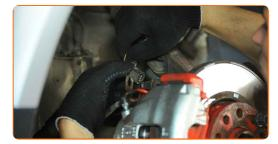
Connect the brake pads wear sensor.
