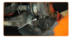
Disconnect the ball joint from the steering knuckle. Use a ball joint puller. Use a hammer.
