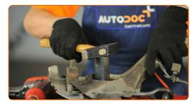
Press out the wheel hub bearing. Use a bush and bearing driver set.
