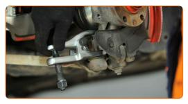
Unscrew the ball joint fastening to the steering knuckle. Use a drive socket #18. Use a ratchet wrench.
