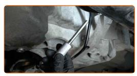
Screw in the TDC timing pin plug. Use a drive socket #E14. Use a ratchet wrench.
