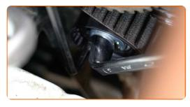
71 Remove the camshaft gear locking tool.
