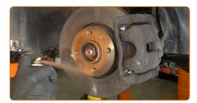
105 Clean the brake disk surface. Use a brake cleaner.
