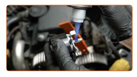
67 Install the timing belt tensioner pulley.
