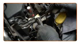
Detach the clamp of the lower coolant pipe. Use long round nose pliers.
