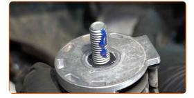
Install the serpentine belt tensioner pulley.
