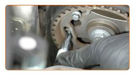
Make a mark on the camshaft gear.
