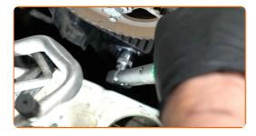
75 Treat the engine mount fasteners. Use a sealant.
