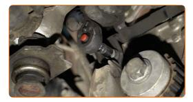
Unscrew the fastener of the serpentine belt tensioner pulley. Use a combination spanner #13.
