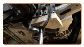
Clean the subframe fasteners. Use a wire brush. Use WD-40 spray.
