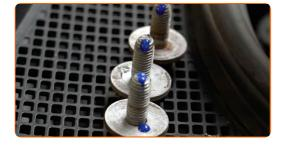
Tighten the upper fastener of the engine mount. Use a drive socket #16. Use a torque wrench. Tighten it to 76 Nm torque.
