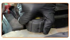
Check the coolant level. If necessary, top up to the required level.
