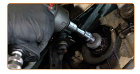
Install the crankshaft pulley according to the factory marks.
