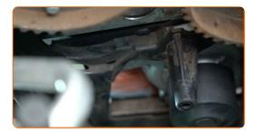
Screw in the fasteners of the middle timing cover. Use a drive socket #8. Use a ratchet wrench.
