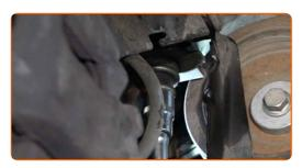
99 Install the fuel filter fastening bracket.
