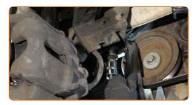
Tighten the subframe reinforcement bracket fasteners. Use a drive socket #13. Use a torque wrench. Tighten it to 35 Nm torque.
