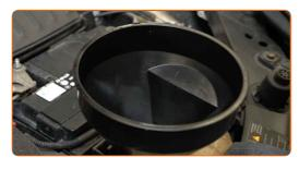
Pour coolant in the coolant reservoir.
