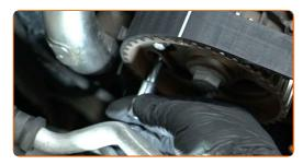
Remove the crankshaft gear locking tool.
