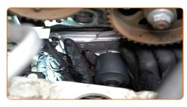
Tighten the water pump fasteners. Use a drive socket #8. Use a torque wrench. Tighten it to 12 Nm torque.
