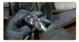
Unscrew the subframe fastening. Use a drive socket #18. Use a ratchet wrench.
