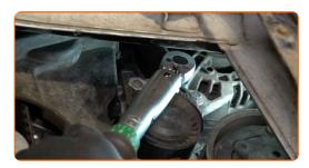
Unscrew the crankshaft pulley fastener. Use a drive socket #18. Use a ratchet wrench.
