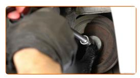
Remove the crankshaft pulley.
