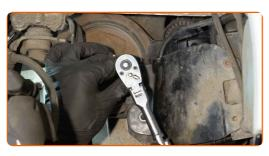
103 Install the wheel arch cover to its mounting seat.
