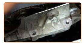
Tighten the engine mount fastening bolts. Use a drive socket #10. Use a torque wrench. Tighten it to 40 Nm torque.
