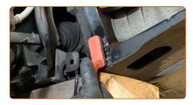
Unscrew the subframe reinforcement bracket fasteners. Use a drive socket #13. Use a ratchet wrench.
