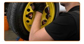
Remove the hub bearing protection cap. Use a hammer. Use a crowbar.
