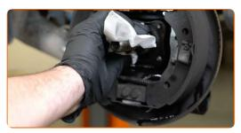
Apply special grease to the bearing assembly mounting seat. Use a multipurpose grease.
