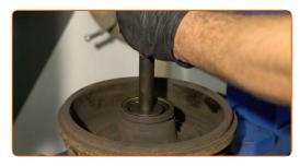
Clean the hub bearing mounting seat. Use WD-40 spray.
