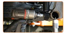
10 Remove the fastening bolt.
