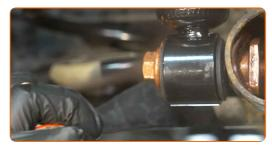
Connect the ABS sensor wiring.
