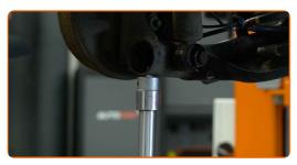
Unscrew the lower fastener of the shock absorber. Use a drive socket #18. Use a ratchet wrench.
