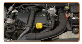
Check the oil level 5 minutes after the stop of the engine operation using a dipstick and add oil if necessary.
