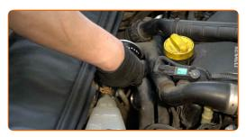
Screw the new filter into its place. Use the 76-14F socket. Use a torque wrench. Tighten it to 25 Nm torque.
