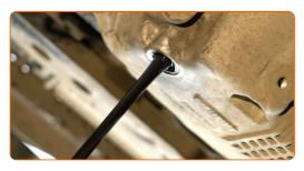
Replacement: engine oil and filter – Renault Clio 3. Tip from AUTODOC:
