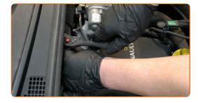
Remove the fender protection cover.
