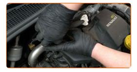
Attach the engine wiring harness. Use a flat screwdriver.
