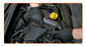
Fasten the clamp on the air intake hose. Use combination pliers.
