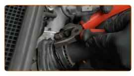
Remove the air intake pipe.
