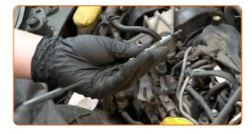
Treat the glow plugs. Use the injector & glow plug grease.
