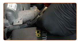
Unscrew the engine cover fastener. Use a drive socket #10. Use a ratchet wrench.
