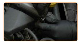
Detach the air intake hose clamp. Use combination pliers. Use a crowbar.
