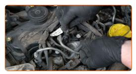
Unscrew the glow plugs. Use the spark plug socket #10. Use a ratchet wrench.
