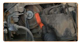
Unscrew the fuel filter bracket fixing bolts. Use a drive socket #13. Use a ratchet wrench.
