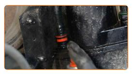
Remove the fuel filter fastening bracket.
