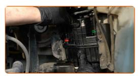
Screw the fixing bolts of the fuel filter bracket. Use a drive socket #13. Use a torque wrench. Tighten it to 19 Nm torque.
